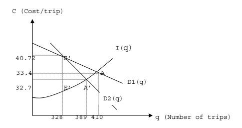
Point A is the 2005 pre-toll situation, with q=410 and c=I410)=33.36. Point B' is the 2006 post-toll situation, with q=328 and c=I(328)+E'B', with the toll E'B'=9.7, ie with c=40.72
